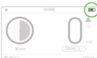
Figure 40. Battery charging indicator
